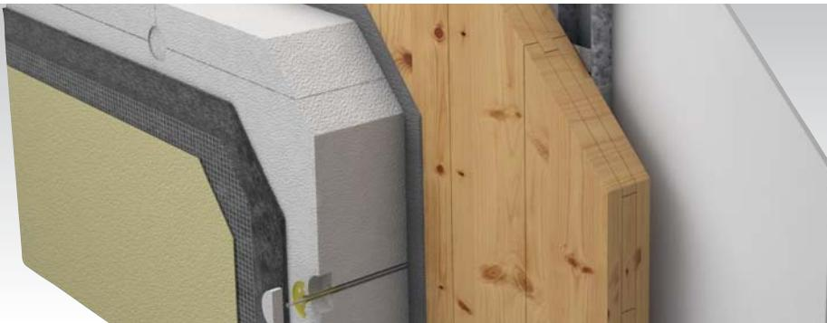
NOSNÁ OBVODOVÁ STĚNA Z KONSTRUKČNÍHO PRVKU DEKPANEL D 81 F, OPATŘENÁ Z EXTERIÉRU VNĚJŠÍM KONTAKTNÍM ZATEPLOVACÍM SYSTÉMEM (ETICS). Z INTERIÉRU JE NA PANELU SÁDROKARTONOVÁ PŘEDSTĚNA NA KOVOVÉ NEBO DŘEVĚNÉ KONSTRUKCI.
